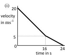
8. While driving along a motorway a driver spots an accident and brakes. The graph below represents the motion of the car from the instant the driver sees the accident.
