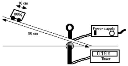
The mass of the trolley is 800 g and it has a length of 10 cm.
