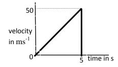
14. How far does a golf ball travel if the velocity - time graph for its flight is as shown below.
