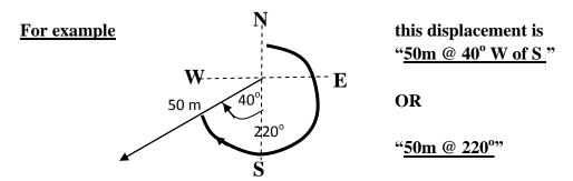
Describe each of the following displacements using appropriate compass points <u>and</u> with a three figure bearing.
